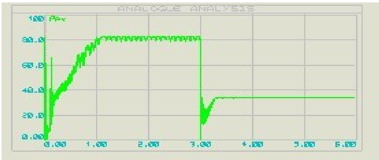
Fig.7. Curve of Temporal Variation of the Power provided by the PV Panel used in the modelled PV system (Fig. 3). This curve is obtained in case where the insolation takes the value G1 = 1000 \text{ Watt/m}^2 and then the value G2 = 364 \text{ Watt/m}^2 after a period of time
